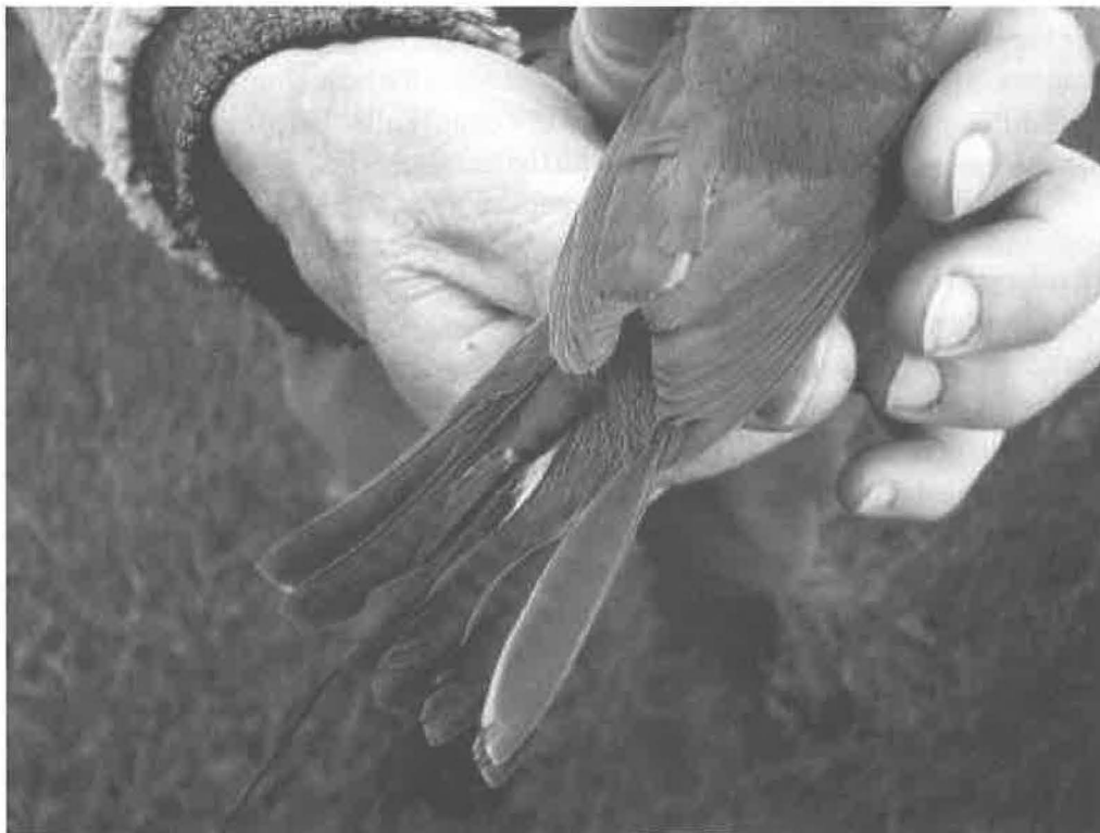
Fig. 2. This shows a transmitter on a chat after heat was applied via 35-watt soldering iron. Note how tightly wrapped the tubing is around the transmitter.
