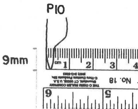
**Fig. 1b.** No. 18 clear plastic rule used to measure P10 and P9 widths at 9 mm from the primary tip.
