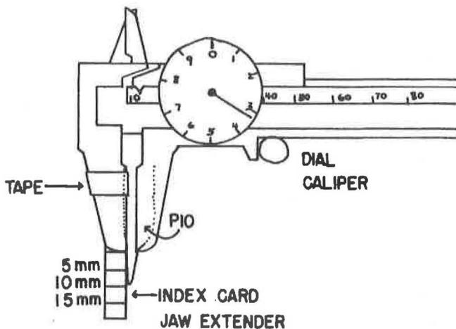
**Fig. 1a.** Dial caliper as modified with extender on left jaw to measure primary tip width of Eastern Kingbirds at 5, 10, and 15 mm. It is shown here superimposed over P10, measuring at 10 mm from the primary tip.
