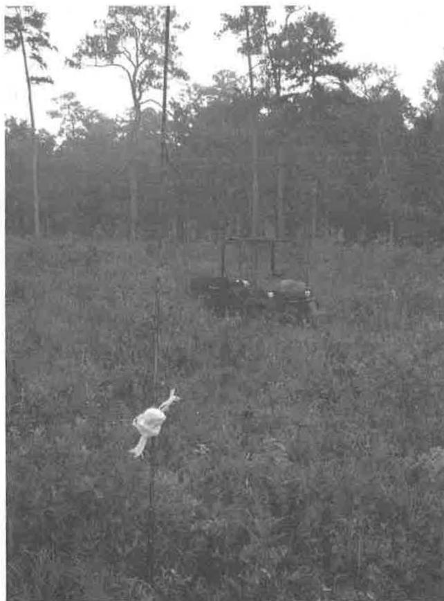
**Fig. 3. Off-road vehicle with base poles attached to the front frame. Another base pole is attached to the tailgate but is not deployed in this picture. The white object in the seat is a CD player, and the plastic grocery bag used to store nets is wrapped around the front net pole in this picture.**
