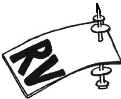
Fig. 2. The tag and pin unit. When intact, from the inside out: pin head glued to plastic washer, soft washer, bird wing, tag, soft washer, plastic washer.
