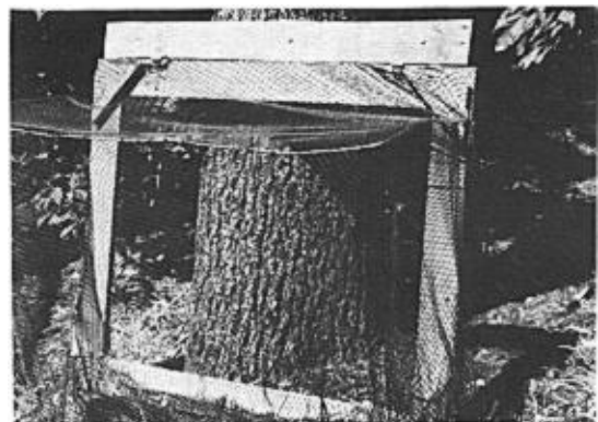
Figure 4A. Catch window: Window in position for trapping, the outside dimensions of the wood frame are 114 x 86 cm, the wire net support extends 55 cm from the frame, and the net sock is 3.4 m long.
