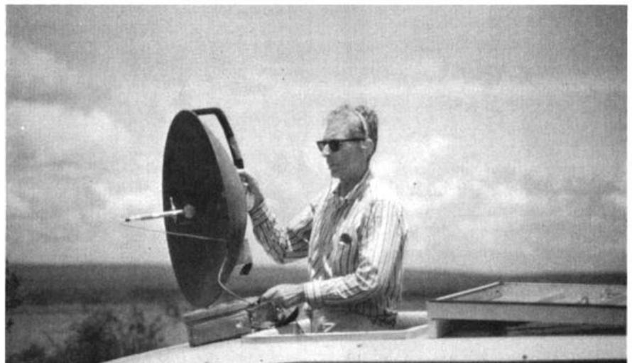
William W. H. Gunn using a parabolic reflector and tape recorder in the field.
