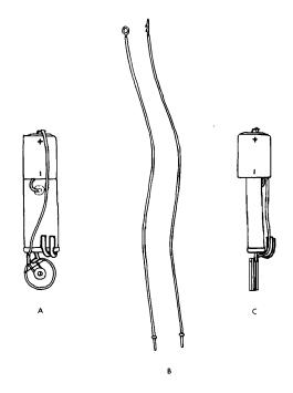
Figure 1. A and C: Bottom and side views of transmitting device; B: Primary lead and reference lead.
