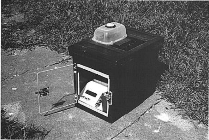
FIGURE 1. Weatherproof field box with electronic balance.
