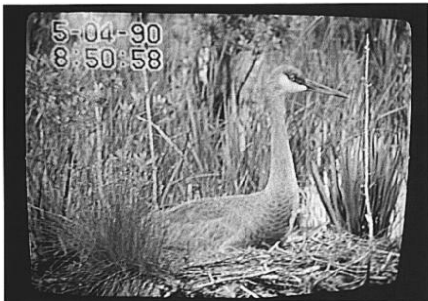
FIGURE 6. Video monitor display showing an adult crane incubating. The camera lens is zoomed in approximately one half for the picture shown. The date (month-day-year) is in the top upper left with time (24-h clock) below. The date and time are recorded continually on the video tapes exactly as shown. The image on the monitor screen is actually much sharper than shown by a photograph of the screen.
