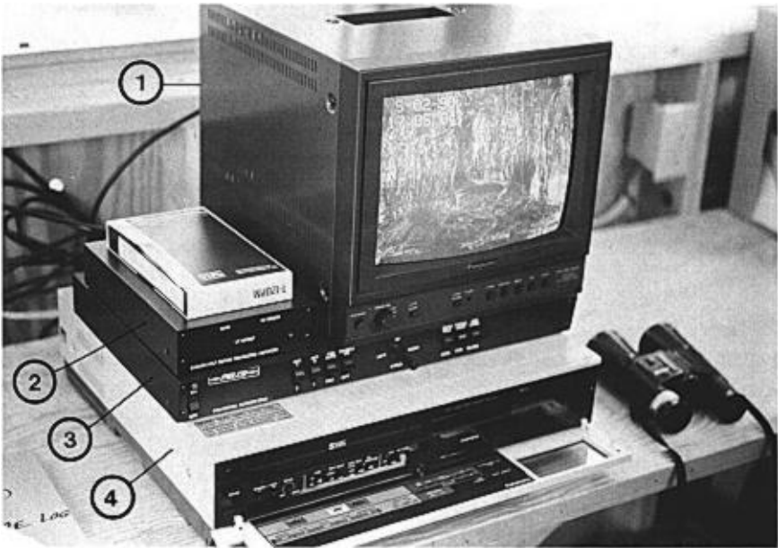
FIGURE 2. The control, monitoring and recording equipment for the CCTV system consists of: (1) color video monitor with incubating crane displayed on screen, (2) half-duplex equalizing amplifier, (3) Coaxitron System 2000 transmitter-controller and (4) time-lapse video cassette recorder.
