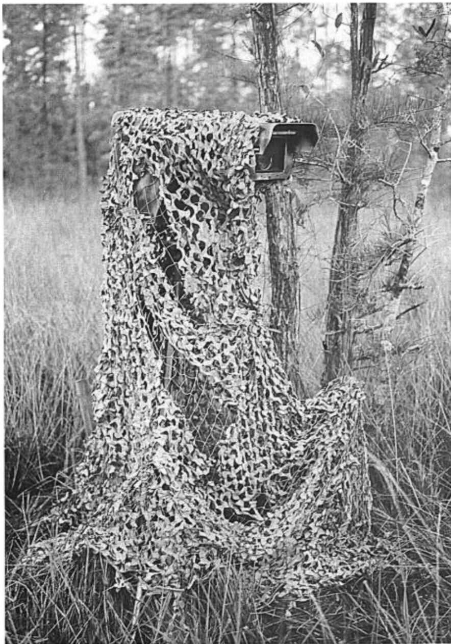
FIGURE 1. CCTV camera setup in the field at a Mississippi Sandhill Crane nest (before installation of infrared illuminator). The unit is draped with camouflage netting and placed near existing trees and shrubs wherever possible to make it less conspicuous.
