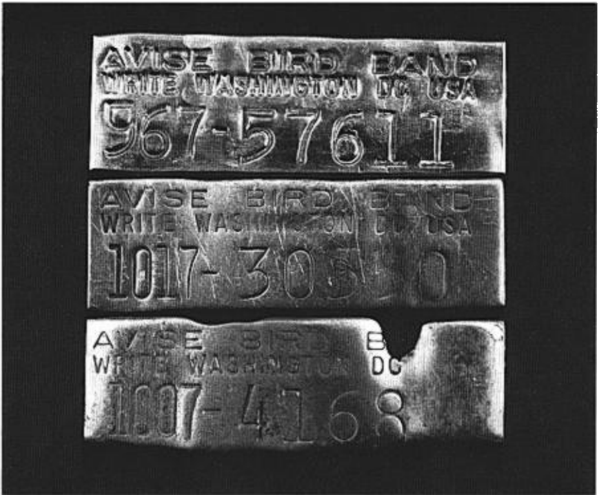
FIGURE 5. Top—New band. Middle and Lower—Differential wear and sinusing of bands caused by poor rotation on the tarsus. Note lower band was placed upside down on the tarsus.
