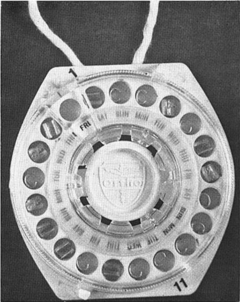
FIGURE 1. Reusable cassette holder for small butt-end aluminum bands.
