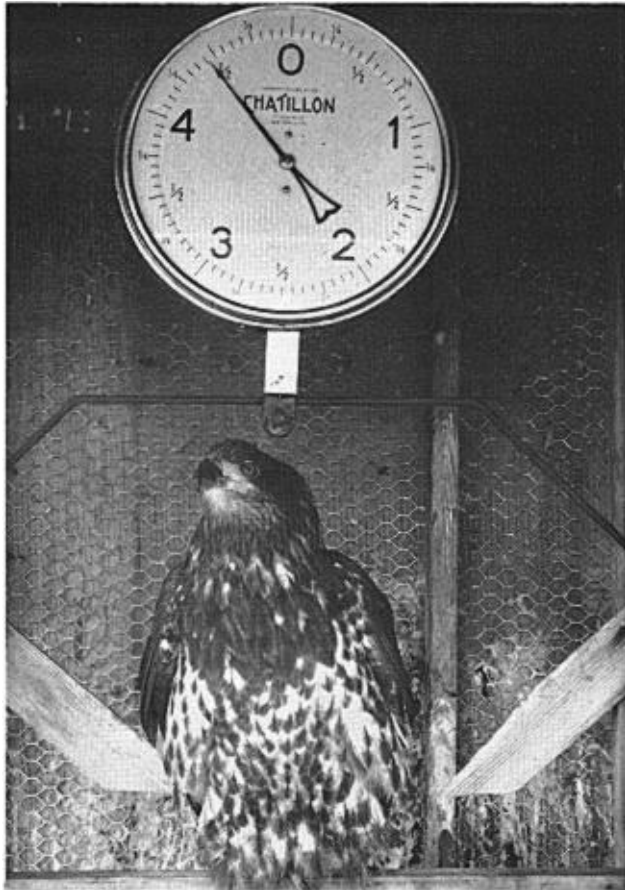
Figure 1 Combination roosting and weighing perch for Bald Eagle. The hand of the balance has made one revolution for 5 pounds which is not shown on the photograph.
