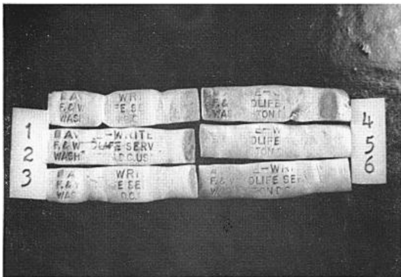
PHOTOGRAPH 1. Crease wear in Aluminum Bands worn by Ring-Billed Gulls. These are six size 5 Short Aluminum Bands which had the address printed on the inside of the band. All bands were worn 4.92 years.
