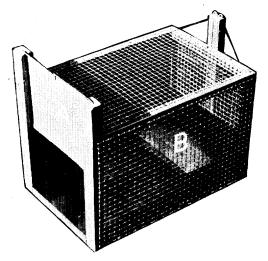
Made of 3 mesh wire  $8'' \ge 12'' \ge 8''$ Automatic balanced feed-tray (B) releases door (A).
