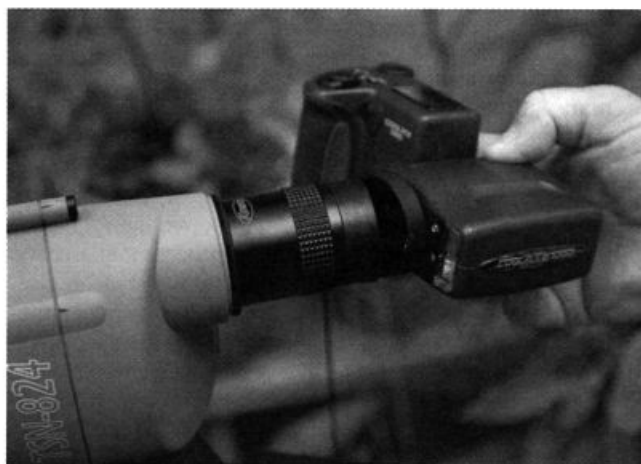
Fig. 4. Author's digiscope equipment showing modified dust cap connector on camera lens slipped onto scope eyepiece (rubber to rubber).
