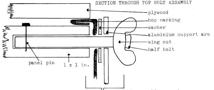
protrudence from 1 x 1 has to be enough for hop sacking, washer, width of aluminium strip and a certain amount of movement of the wing nut along the bolt, approx 1 inch.
