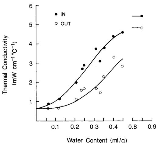
FIGURE 2. Thermal conductivity ( $\text{mW cm}^{-1} \text{ } ^\circ\text{C}^{-1}$ ) of Brush-turkey mound material as a function of water content (ml/g dry material). The two curves were fitted by eye to data obtained when heat was moving inward (●) or outward (○) through a cylinder of the material.
