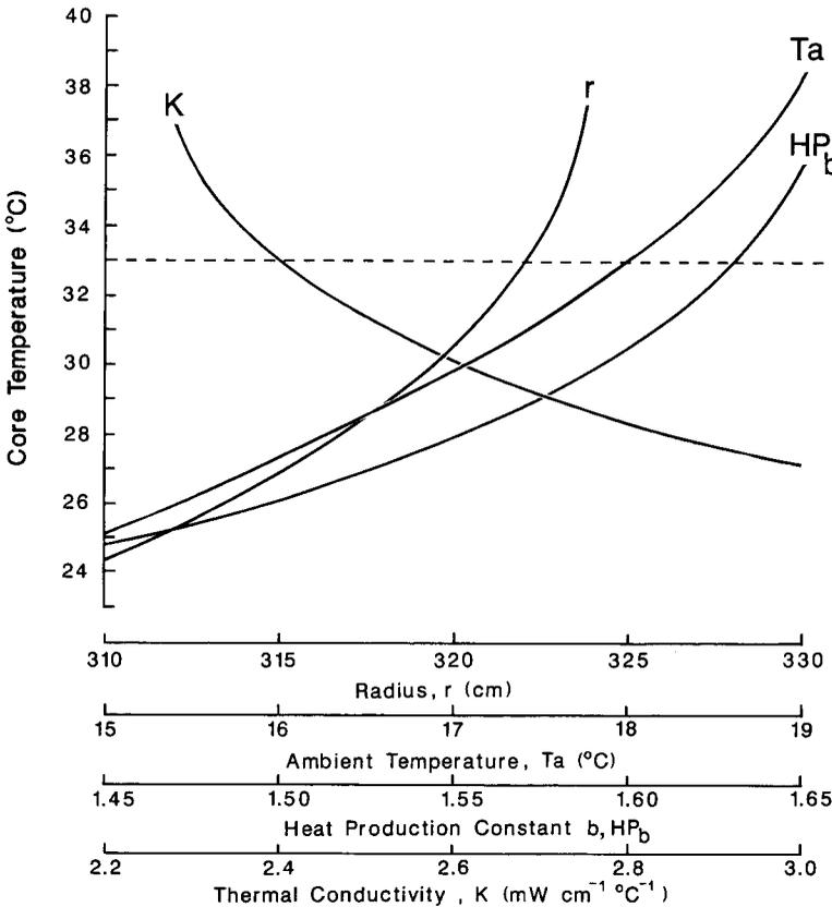
FIGURE 7. Effect of changing selected parameters on equilibrium core temperature in the numerical model of a Brush-turkey mound. All parameters are fixed at "standard conditions" except those under investigation (see text). Dashed line represents observed average core temperature of 33°C.
