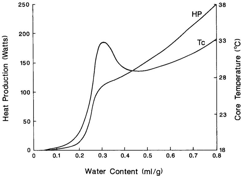
FIGURE 8. Effect of water content (ml/g dry material) on equilibrium core temperature ( $T_c$ ), and total rate of heat production (HP), in the lens-shaped active zone of our model Brush-turkey mound (Figure 1).
