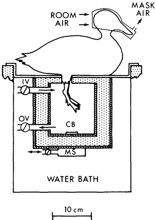
FIGURE 1. Cross-sectional view of calorimeter positioned within the refrigerated water bath. Circulation of fluid through the calorimeter bath (CB) was controlled by the inlet (IV) and outlet (OV) valves. The magnetic stirrer (MS) was air driven. Room air was drawn through the mask fitted over the duck's head.
