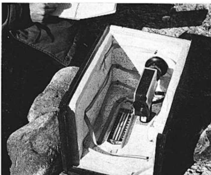
Figure 2. Insulated box with heat tape housing 8-mm Braun-Nizo S-80 camera.
