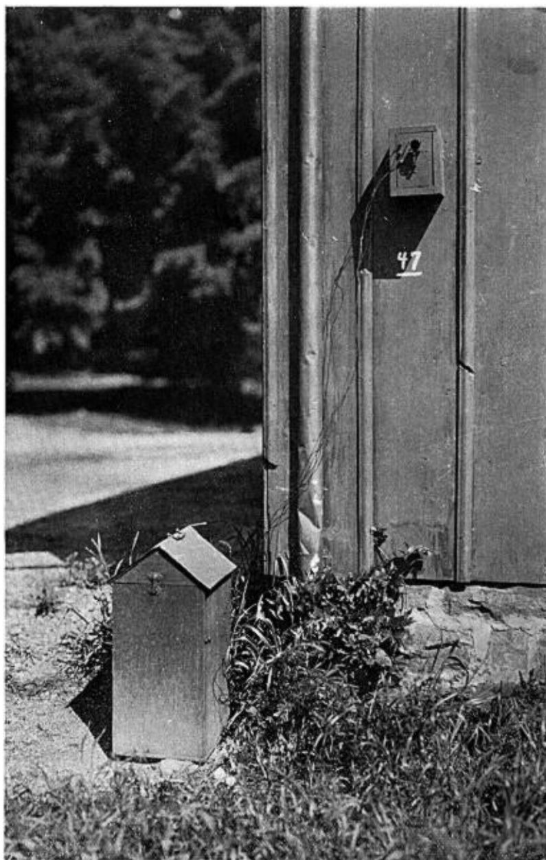
Clock itograph in weather case (closed) and set up below wren box, to which it is connected by wires.
