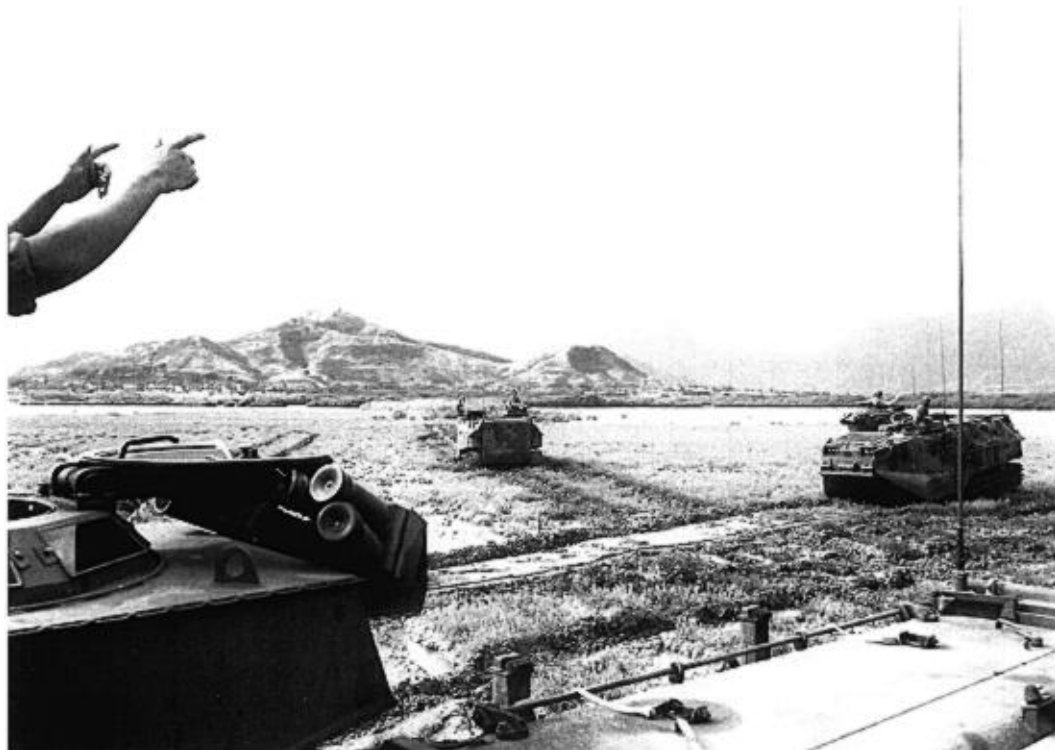
FIGURE 3. Marine amphibious assault vehicles plowing mudflats of Nu'upia Ponds, crushing invasive weeds, and opening water channels to expand and improve Hawaiian Stilt nesting and feeding opportunities. (Photo by D. Drigot).
