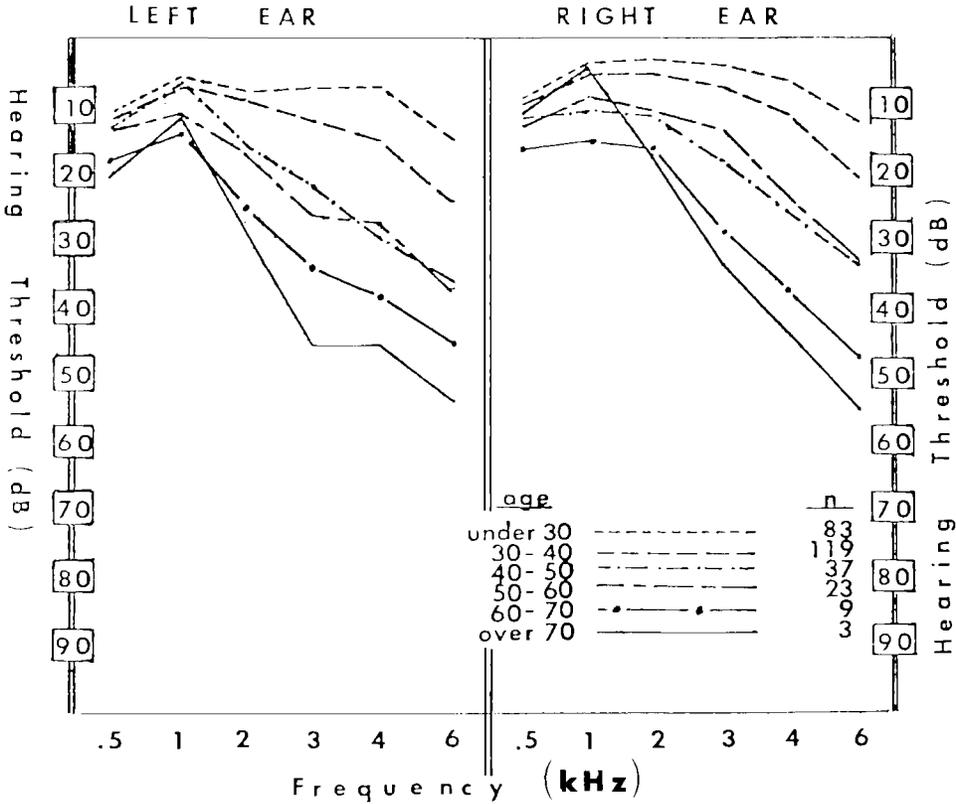
FIGURE 1. Age profiles of average hearing thresholds over the frequency range 0.5 to 6.0 kHz.
