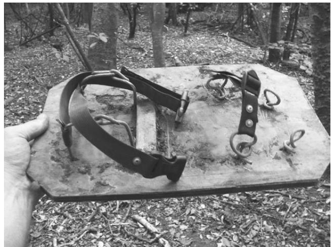
**Fig. 2.** Early petrel board design using wire-and-strap bindings with a wooden instep locator. Many variations of these easily fashioned and relatively durable binding materials were tried. *Photo: E. Kennedy*
