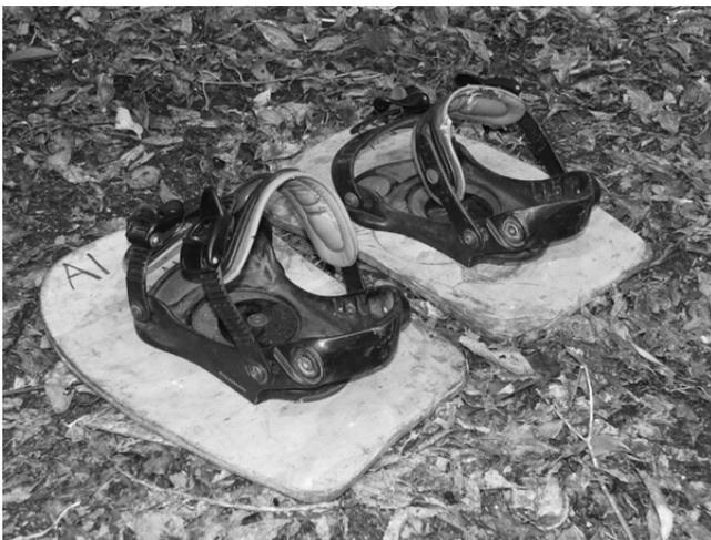
**Fig. 1.** Current petrel board design using commercial snowboard bindings to accommodate standard field footwear. *Photo: E. Kennedy*
