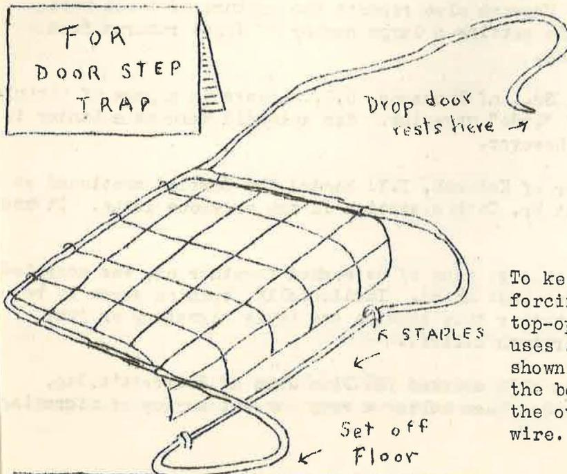
Mr. Baily uses several traps with a wooden floor both on the ground and hung in trees. In place of the conventional door-step trigger, he uses a trigger as shown.
