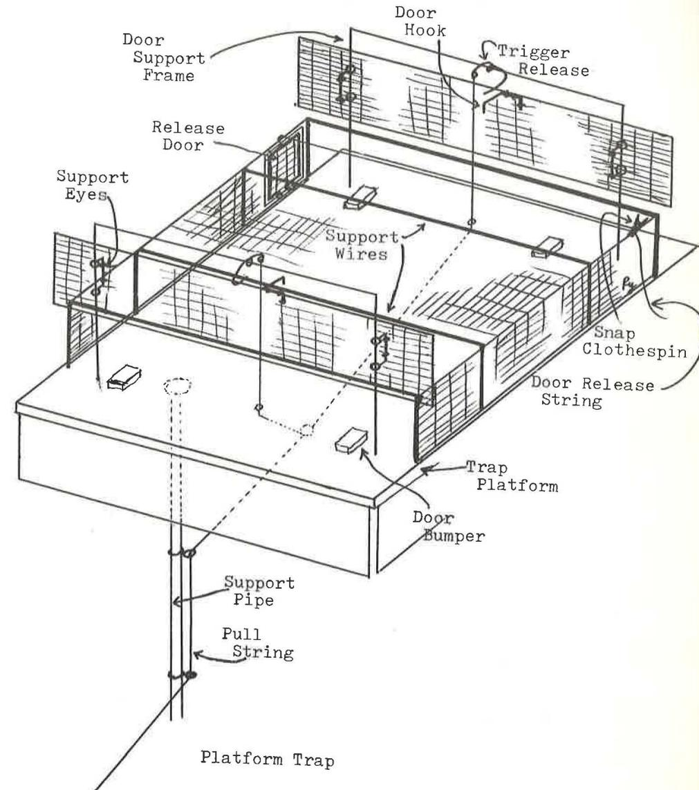
The open ended cage is typically eight in. high, and the two I use presently measure 32 inches wide by 30 in. deep, and 36 in. wide by 34 in. deep. The cage is supported by three or four support wires made of 9-gauge galvanized wire. These wires are squeeze fitted into holes in the platform to anchor the trap in place.
