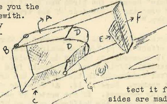
This trap is 8" wide by 8" high and is 16" long. The bottom and end "F" is solid wood 1" thick to protect it from snow. The top and sides are made of hardware cloth without a frame as the bottom and end will give sufficient support. Possibly glass would be better than the hardware cloth.
