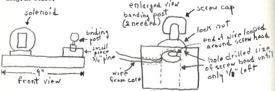
Next a control button is assembled to trip the solenoid. This can be an ordinary door-bell button. The button is assembled in a small box with a cord to plug into 110 volts on one side and again two binding posts on the other side. See diagram below.
