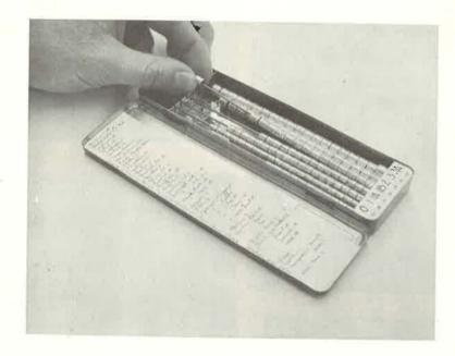
It is made from a steel pencil-box with a hinged lid. A block of wood into which 1/16 inch diameter brass rods have been inserted is glued in the lower end. The rods are cut short enough so a finger can be placed between the ends of the rods and the end of the pencil-box to spring the desired rod high enough to permit removal of a band. The free ends of the rods rest in grooves filed in a piece of thin sheet metal bent at right angles and soldered to the pencil-box. These grooves
