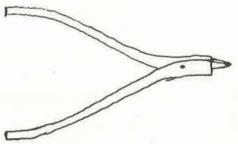
Bands are opened by inserting the point in the band and squeezing the handles.
