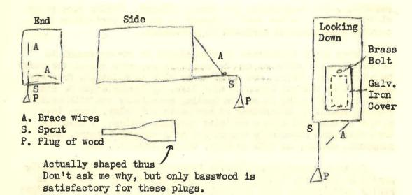
I formerly used a "screw on" cap and soldered the drip wire into it. Mostly I now use the one sketched here and shown in the photo so I don't have to remove the can to fill it. I cut a rectangular hole in the top about 1-1/2 x 3" and place a cover slightly larger over this to keep out mice, bugs and trash. This cover is pivoted on a brass bolt at one end.
