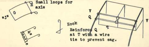
A handle for the door and hooks on the bottom, on each side of the door, are easily installed and are made of heavy wire.
