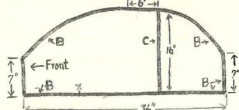
STEP ONE: - Make 2 frames as above exactly alike of No. 9 galvanized wire. "B" is one piece of wire joined at "X". "C" is a separate piece of wire. See detail below for connections.
