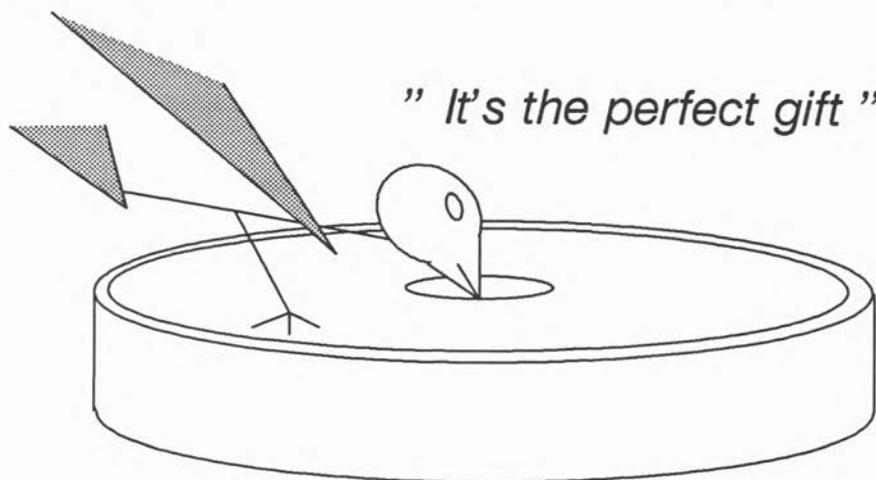
The bird-tested SOLAR SIPPER uses the power of the winter sun to extend the time that water remains liquid in freezing temperatures during daylight hours.
