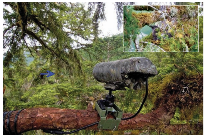
Fig. 1. Photo showing placement of a zoom lens relative to the Hemmingsen Creek Marbled Murrelet nest in 2006 (nest is indicated with arrow), on Vancouver Island, British Columbia. Zoom lenses were typically placed in nearby trees on limbs 30–50 m from the nest. A ~50-m cable extended from the lens to the ground. Deep-cycle batteries (for powering the camera) and a digital video recorder (for recording and storing video files) were placed on the ground below the camera tree. Thus, when we visited the nest to replace batteries we did not have to climb the camera tree. Inset photo in upper right shows the Hemmingsen Creek Marbled Murrelet incubating an egg on the nest. Photos by N.R. Hatch.
