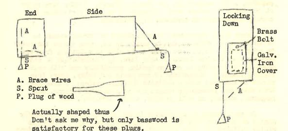
I formerly used a "screw on" cap and soldered the drip wire into it. Mostly I now use the one sketched here and shown in the photo so I don't have to remove the can to fill it. I cut a rectangular hole in the top about 1-1/2 x 3" and place a cover slightly larger over this to keep out mice, bugs and trash. This cover is pivoted on a brass bolt at one end.
